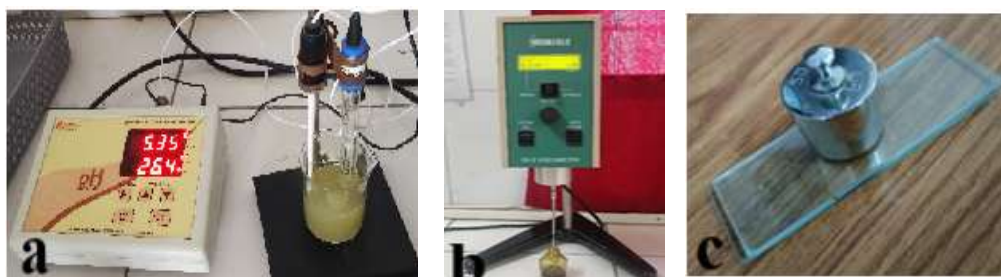
Figure 1D: Determination of evaluation parameters of herbal serum (a) pH meter, (b) Brookfield viscometer, (c) Spreadability
